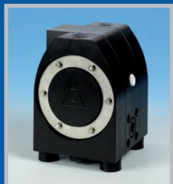
The heavy-duty muffler in the center housing is made of expanded PE (the conductive versions of E 15 – E 50 are equipped with a bronze one). Direct installation of the stationary pumps is facilitated by shock absorbers with female thread on the underside. The positions of the connections are corresponding to those of the predecessor A-Series.
